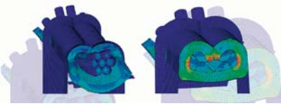
Crimping of wires Courtesy of TYCO Electronics
